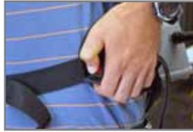
On-Off Switch: Hip mounted for easy access.
