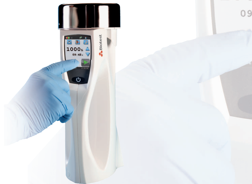
Fig. 2: Main window for volume selection and activation of sampling at the touch of a button
