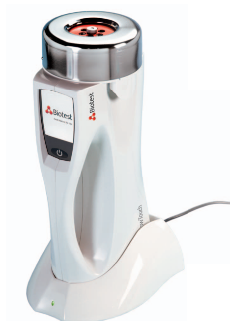
Fig. 4: LED-controlled docking station for easier charging of the integrated battery
