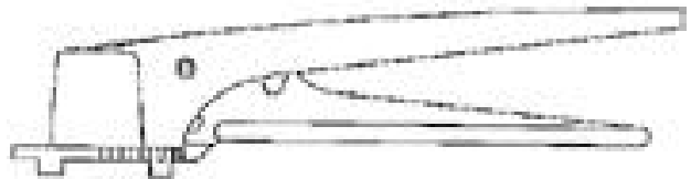
Fig. 8. LKB lockable multi-position handle
