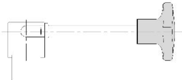
Fig. 7. LKB butterfly valve regulating handle
