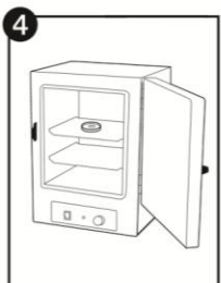
4. Incubate at 37^{\circ} \pm 0.5^{\circ}\text{C} for 6 hours for quantitative measurement or 8 hours for qualitative measurement. This is the enriched sample. Proceed to Step 2.
