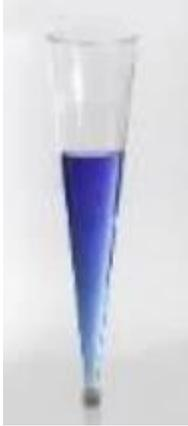
Made for measuring sand and other settled matter in water and sewage, these Imhoff cones are molded of glass-clear, unbreakable styrene acrylonitrile. Use a Poxymat® cone rack to support three or four Imhoff settling cones in a single row for clearer viewing.
