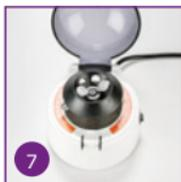
7 Centrifuge the diluted sample extract for 30 seconds. Take the supernatant for further testing.
