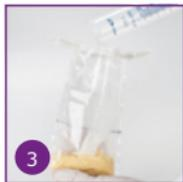
3 Add 50 ml of distilled water to Whirl-Pak® filter bag.
