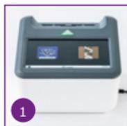
1 Turn on the AgraVision™ Pro reader by plugging it in and follow the set up procedure according to the instructions.
