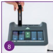
8 Insert the AgraStrip® Pro test strip into the AgraVision™ Pro cartridge. Transfer the cartridge containing the test strip into the port of the reader.
