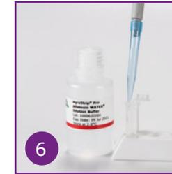
6 Pipette 1000 µL assay dilution buffer into a microcentrifuge tube.\*
