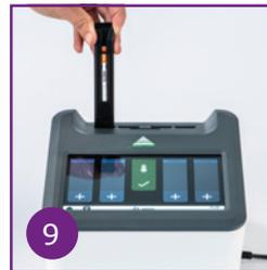
9 Insert the test strip into the provided cartridge. Place the cartridge containing the test strip into a reader port.
