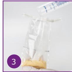
3 Add 50 ml of distilled, deionized or bottled water to the Whirl-Pak® filter bag.
