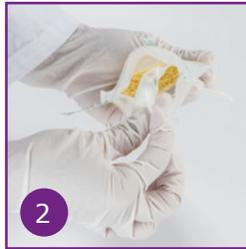
2 Weigh in 10 g of adequately ground, representative sample into one side of a Whirl-Pak® filter bag. Add one extraction buffer bag into the same side.
