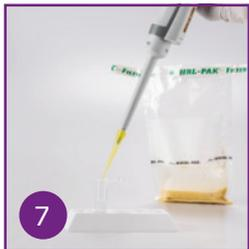
7 Transfer 100 µl of sample extract supernatant from the filter bag to the microcentrifuge tube (1:11 dilution).\*
