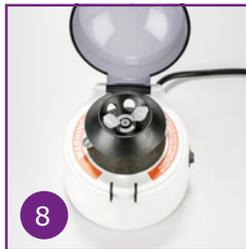
8 Centrifuge the diluted sample for 30 seconds at 2000 g.
