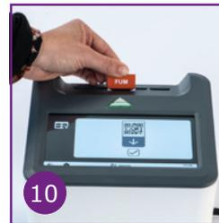
10 Insert the QR card containing information the reader needs to carry out the test. Once saved, it will not need to be scanned again.
