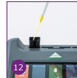
12 Pipette the sample extract into the cartridge. The reader automatically starts the assay and displays the result when finished.
