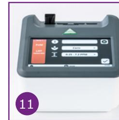
11 The AgraVision™ Pro detects the test strip via the data matrix code on the strip. Enter sample ID, matrix type and quantitation range.
