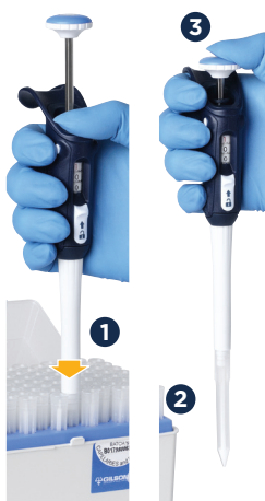
Figure 4 CP fitting on MICROMAN® E
