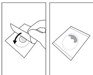
**4** Roll the top film down onto the sample.
