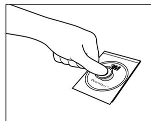
**6** Press firmly on the center of the spreader to distribute the sample evenly. Spread the inoculum over the entire 3M Petrifilm Rapid Yeast and Mold Count Plate growth area before the gel is formed. Do not slide the spreader across the film.
