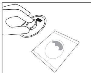
**5** Place the 3M™ Petrifilm™ Flat Spreader (6425) or other flat spreader on the center of the 3M Petrifilm Rapid Yeast and Mold Count Plate.
