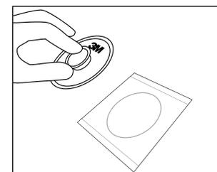
**7** Remove the spreader and leave the 3M Petrifilm Rapid Yeast and Mold Count Plate undisturbed for at least one minute to permit the gel to form.
