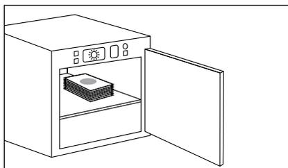
**8** Incubate 3M Petrifilm Rapid Yeast and Mold Plate at 25°C ± 1°C or 28°C ± 1°C for 48h ± 2h in a horizontal position with the clear side up in stacks of no more than 40. Please refer to the product instructions for third party validated methods.
