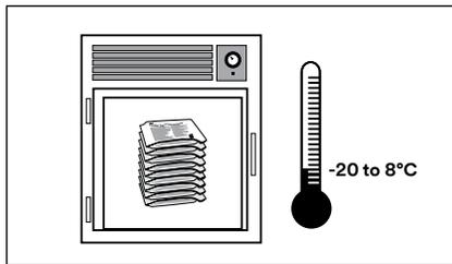
**1** Store the unopened 3M Petrifilm Rapid Yeast and Mold Count Plate pouches at frozen or refrigerated temperature equal to -20 to 8°C (-4 to 46°F). Use before expiration date on package. It is best to allow pouches to reach room temperature before opening.
