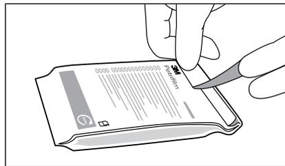
**2** Seal by folding the end of the pouch over and applying adhesive tape. To prevent exposure to moisture, do not refrigerate opened pouches. Store resealed pouches in a cool dry place (20–25°C / <60% RH) for no longer than four weeks.
