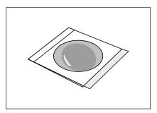
Gently roll down the top film onto the diluent to prevent trapping air bubbles.
