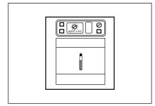
8 Incubate the R-V R10 at 41.5°±1°C for 8–24 hours. Move to step 13b after first performing steps 9–12.
