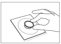
Place the 3M Petrifilm Flat Spreader on the center of the plate. Press gently on the center of the spreader to distribute the diluent evenly. Spread the diluent over the entire 3M Petrifilm Salmonella Express Plate growth area before the gel is formed. Do not slide the spreader across the film.
