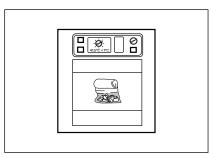
6 Incubate the enriched samples at 41.5°±1°C for 18–24 hours. For low microbial background samples (<10⁴ CFU/g), move to step 13a after first performing steps 9–12.
