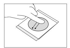
Roll down the top film to close the 3M Petrifilm Salmonella Express Plate. Using a gloved hand (while practicing good laboratory practices to avoid cross contamination and/or direct contact with the plate), gently apply a sweeping motion with even pressure onto the top film to remove any air bubbles in the inoculation area.
