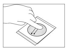
Using a gloved hand, gently apply a sweeping motion with even pressure onto the top film to remove any air bubbles in the inoculation area and assure good contact between the gel and the 3M Petrifilm Salmonella Express Confirmation Disk.
