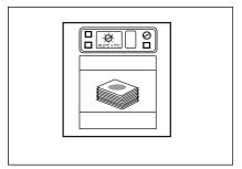
Incubate plates at 41.5°±1°C for 24±2 hours in a horizontal position with the colored side up in stacks of no more than 20 plates.
