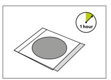
Place 3M Petrifilm Salmonella Express Plate on a flat surface for at least 1 hour at room temperature (20–25°C), protected from light, to allow the gel to form.
