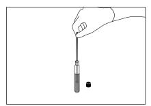
For high microbial background samples, use a sterile 10µL loop to withdraw a full loop of sample for streaking the plate. Use a smooth loop (one that does not have jagged edges and is not distorted) to prevent the gel surface from breaking.
