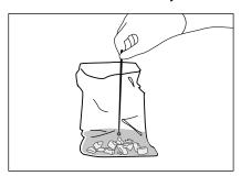
For low microbial background samples, use a sterile 10µL loop to withdraw a full loop of sample. Use a smooth loop (one that does not have jagged edges and is not distorted) to prevent the gel surface from breaking.
