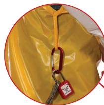
Self-material lock out, tag out (LOTO) straps at each waist
