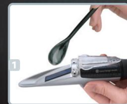
1 Apply 1-2 drops onto the prism.
