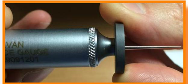
4. Read off the measurement from the dial at the other end of the gauge.
