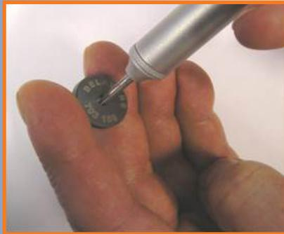
3. Continue to slide the needle into the hole until the flat side of the disc touches the end of the gauge.
