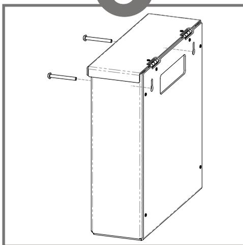
Dispenser should be mounted securely to wall through keyholes in back with screws approved and provided by building maintenance.
