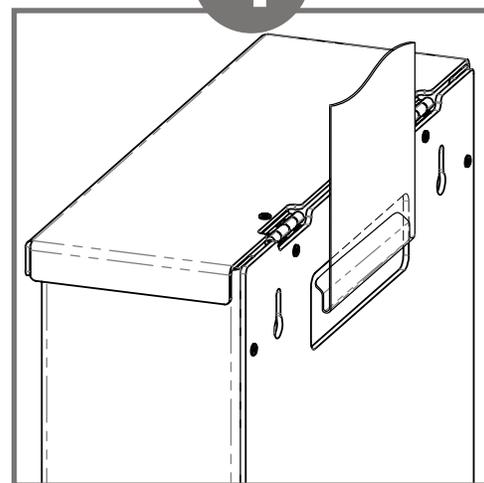
Alternatively, the dispenser can be mounted on a door or wall using a BOWMAN® hanger. Note that dispenser should be mounted to the door or wall *prior* to loading with product.
