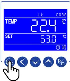
Press the SETTING key to enter the Level 3 controller parameters.
