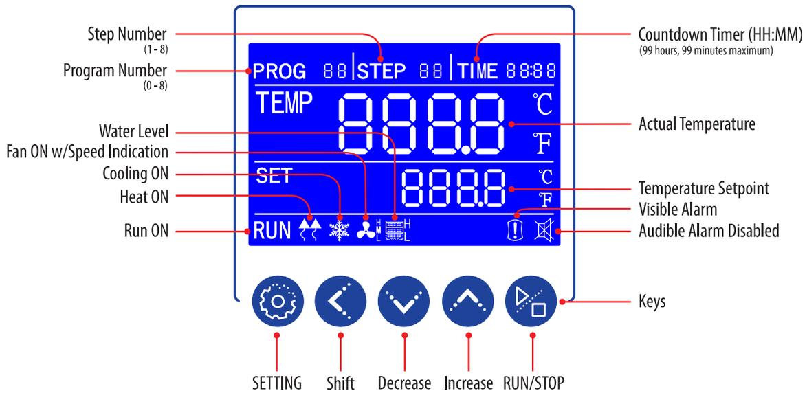
**PROG Area:** Displays the program working or setting group. Controller is capable of programming and storing up to 7 programs.
