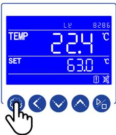
Press the SETTING key to enter the Level 4 controller parameters.
