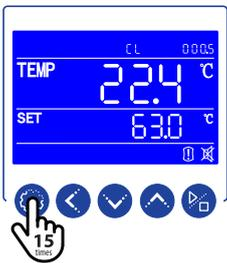
Press the SETTING key 15 times to scroll through parameters until the parameter CF appears.
