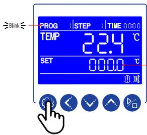
Pressing the SETTING key starts the programming process. STEP 1 will appear. "End" in TIME area will change to run time digits. PROG and the tenths temperature value blinks.
