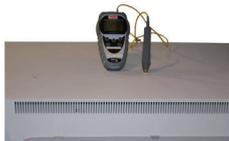
Upon reaching the set temperature, insert thermometer probe into the test hole.
