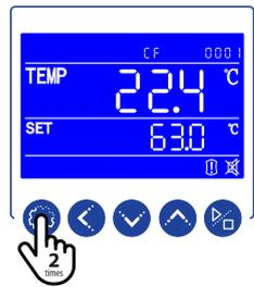
Press the SETTING key 2 times to set parameter CF and return to standard state.
