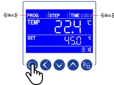
Press the SETTING key to accept temperature setpoint. The first TIME digit will blink.
