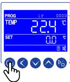
Press the SETTING key to enter Level 1 parameters.
