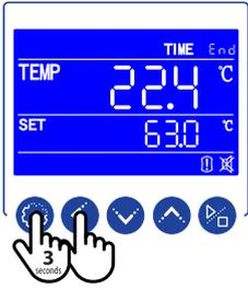
Press and hold the SETTING and shift keys for 3 seconds to enter the controller's internal parameter settings.
