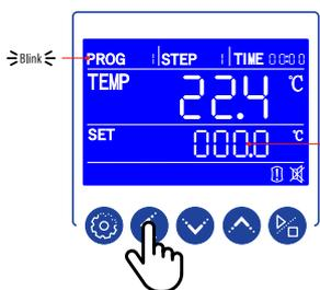
Press the SHIFT key to move to the next parameter digits. Each move will cause parameter to blink.
