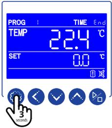
Press the SETTING key for 3 seconds. The "PROG 1" will initially blink. Then the number will blink.
