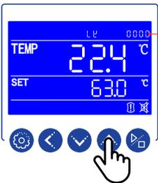
Press the INCREASE key to enter the first code digit. Press the SHIFT key to move to the second code digit. Digit will blink. Press the INCREASE key to enter the second code digit.
