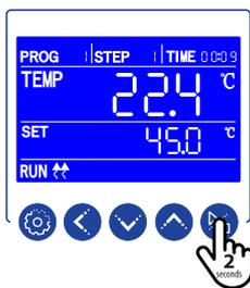
Pressing the RUN key for 2 seconds starts the program. STEP area, RUN, HEAT, and run time illuminate.
