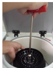
Tool for rotor with nut
