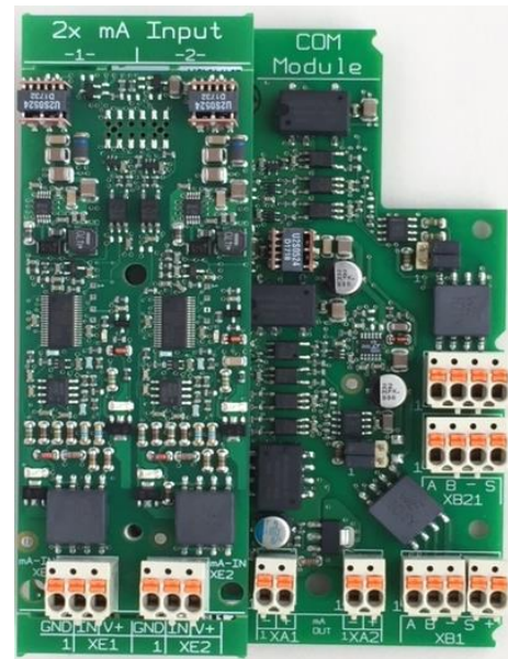
Driver card installed on Com module
