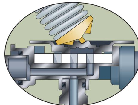
The unique Shuttle Valve creates the ultimate **One of A Kind** performance & reliability. It combines a long life ceramic slide valve with a unique spring design that is stall resistant.
