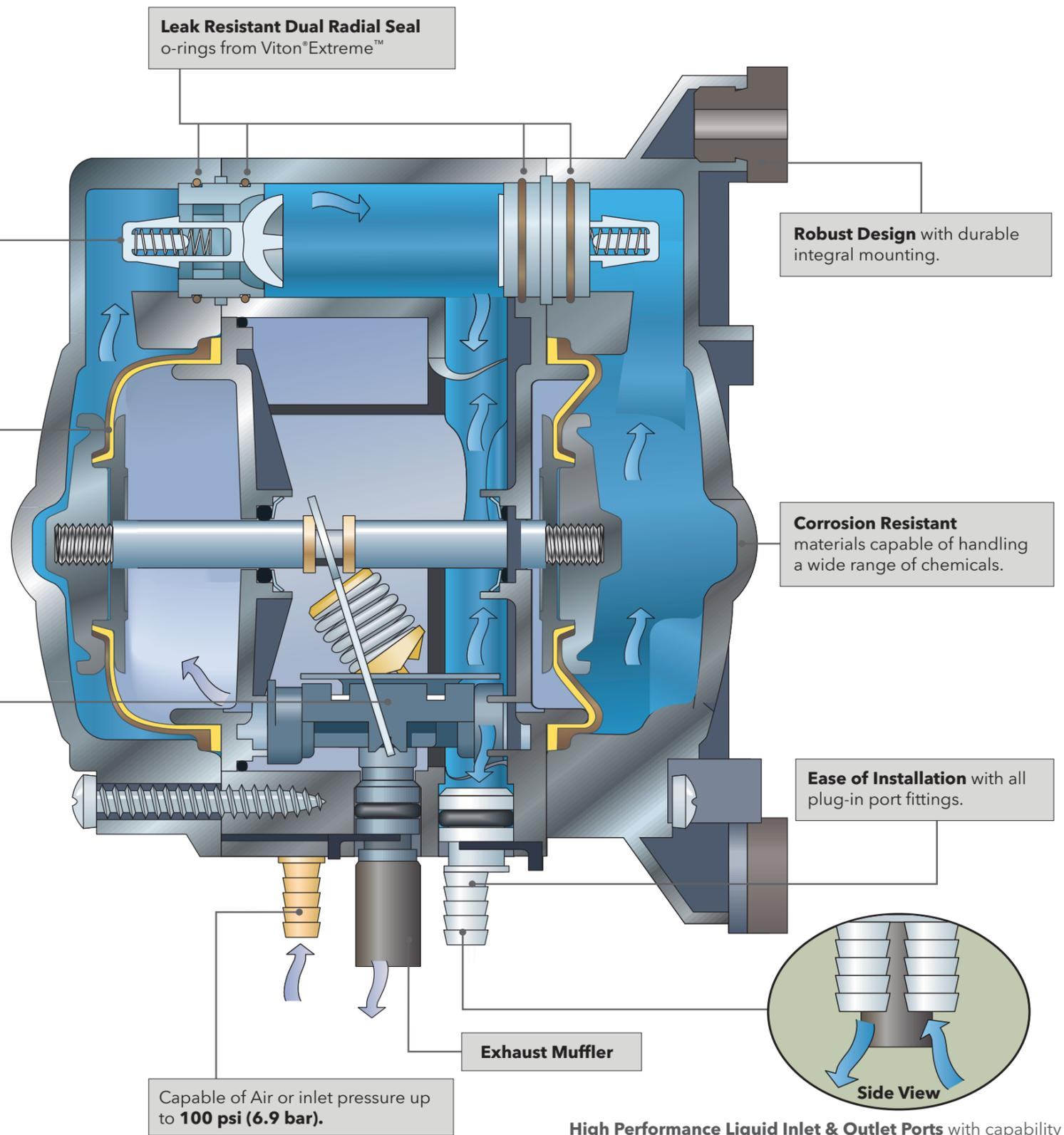
**High Performance Liquid Inlet & Outlet Ports** with capability of supplying flow rate to 5 GPM (18.9 l/min.).
