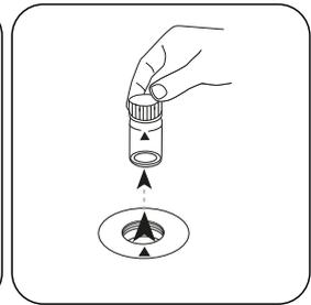
Remove the vial from the sample chamber.
