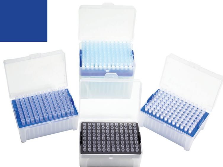
Low retention polypropylene filter tips have a hydrophobic and smooth surface. Polyethylene filter protects against cross-contamination by preventing liquids and aerosols from entering the body of the micropipette. Sterile tips are non-cytotoxic and non-hemolytic. Packaged in racks of 96 with 10 racks in each case, for a total of 960 pieces.
