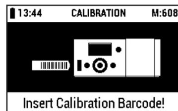
Remove the barcode strip for calibration from the pack (included in the scope of delivery of RQflex® 20).
