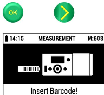
Remove the specific barcode strip from the Reflectoquant® pack. Certain tests require two barcode strips. Insert the barcode all the way into the barcode scanner in the direction of the arrow in a smooth motion from left to right, and then remove it again.
