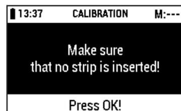
Make sure that no test strip is inserted in the test strip adapter, then press [OK].
