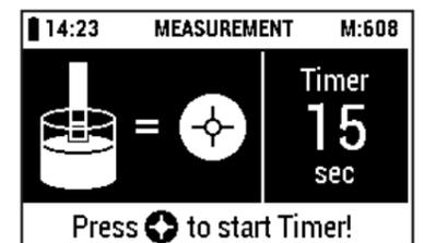
Immerse the test strip into the sample as described in the Reflectoquant® package insert (Reflectoquant® pack) and **at the same time** press the [START measurement] button to start the timer.
