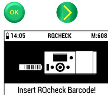
Remove the barcode strip for RQcheck from the pack. Insert the barcode all the way into the barcode reader in the direction of the arrow in a smooth motion from left to right, and then remove it again.
