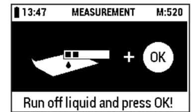
Carefully allow excess liquid to run off via the long edge of the strip onto an absorbent paper towel and press the [OK] button.
