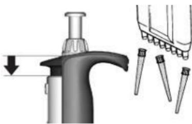
Hold the pipette shaft over a suitable disposal bin and press the tip ejection button all the way down.
