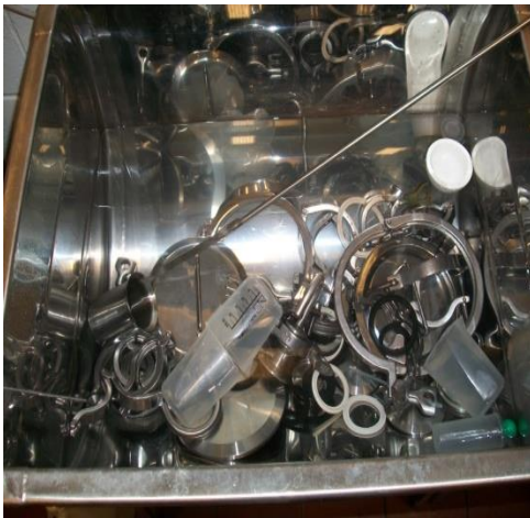
Fig. 18. Incorrect storage of parts in a COP tank. They should be stored in designated areas
