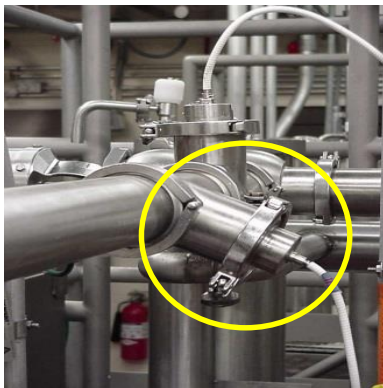
Fig. 15. Accumulation/niche created by reassembling the probe facing down instead of up
