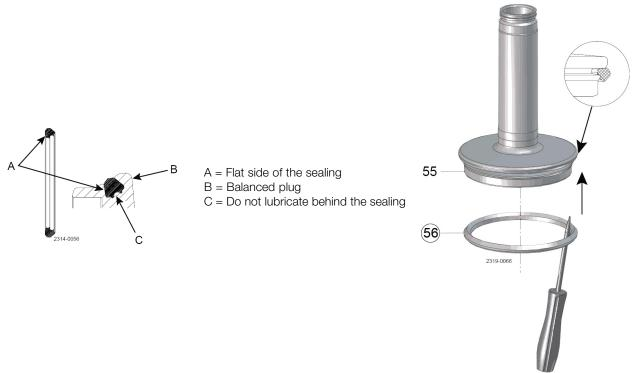
Carefully lubricate sealings with suitable soap or lubricant (Klüber Paraliq GT 703), before pre-mounting.
