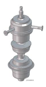
Upper: Balanced with SpiralClean OD balancer Lower: Flush OD Balancer (steel bottom)
