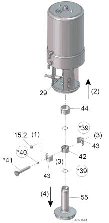
The valve is designed so that internal leakages do not result in the products becoming mixed. Internal leakage in the valve is externally visible.
