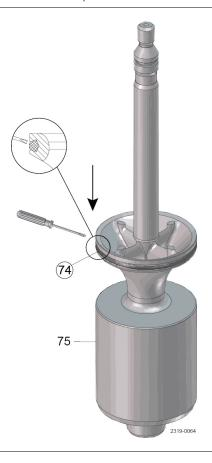
The valve is designed so that internal leakages do not result in the products becoming mixed. Internal leakage in the valve is externally visible.
