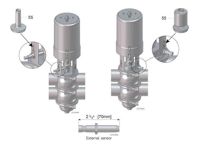
If using external sensor, the sensor must be active/activated when performing a setup routine of the control head.
