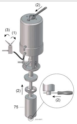
The valve is designed so that internal leakages do not result in the products becoming mixed. Internal leakage in the valve is externally visible.
