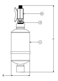
AG1109006 Drain Kit is used on: P-EG 0006-0288 NPT Housing Vent Port P-EG 0006-0288 ANSI Flg Housing Vent & Drain Port
