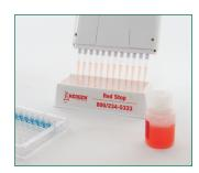
9. Transfer 100 µL Red Stop from reagent boat to antibody wells. Mix.
