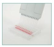
2. Transfer 100 µL to the antibody wells. Incubate for 10 minutes. Mix for 20 seconds by sliding back and forth on a flat surface.
