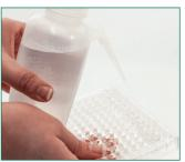
4. Wash wells thoroughly. Repeat wash step wash 10 times times with washing solution.
