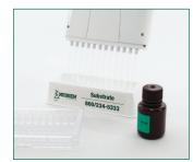
8. Transfer 100 µL substrate from reagent boat to antibody wells using 12-channel pipettor. Incubate for 10 minutes. Mix for 20 seconds by sliding back and forth on a flat surface.
